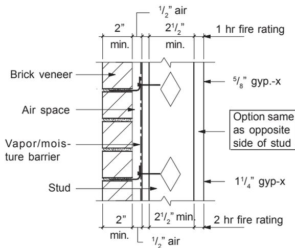
Figure 2 Anchored brick veneer.
