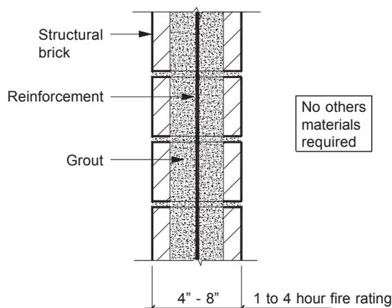
Figure 4 Structural load bearing brick.
