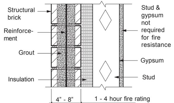
Figure 3 Structural brick veneer.
