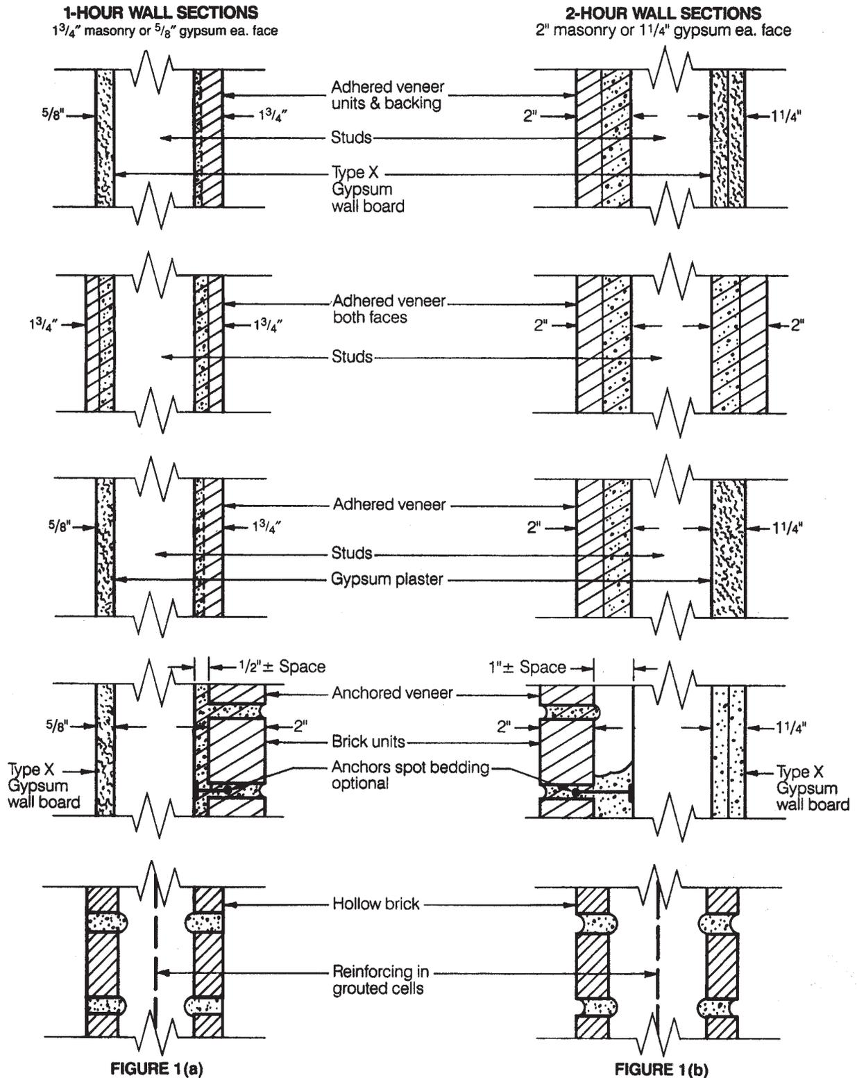
The one-hour walls require not less than 5/8-inch gypsum board or plaster, or 1 3/4 inches of adhered veneer and backing on each face. The two-hour walls require not less than 1 1/4 inches (two 5/8-inch boards) wallboard or gypsum plaster, or not less than 2 inches of brick veneer and backing on each face.
