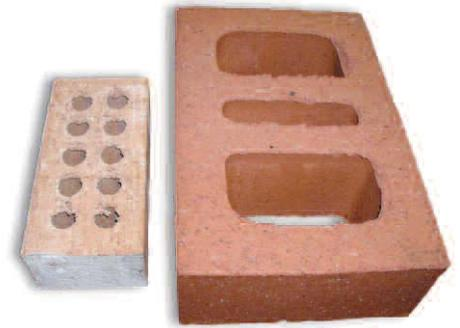
**Solid face brick and hollow structural unit.**
